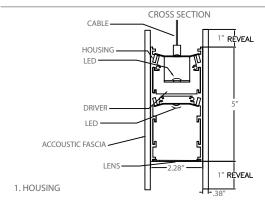
To be formed from 20GA Aluminum Finish: Baked white enamel (standard) Direct / Indirect Lighting (standard) All fixtures pre-wired
