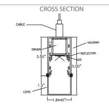
To be formed from 20GA Aluminum Finish: Baked white enamel (standard) Direct / Indirect Lighting (standard) All fixtures pre-wired All steel parts are phosphate treated for corrosion resistance before painting procedure and then baked with superior adhesion for durability
