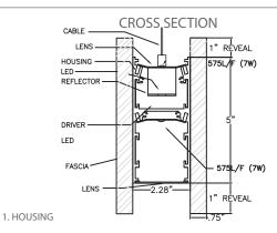
To be formed from 20GA Aluminum Finish: Baked white enamel (standard) Direct / Indirect Lighting (standard) All fixtures pre-wired All steel parts are phosphate treated for corrosion resistance before painting procedure and then baked with superior adhesion for durability
