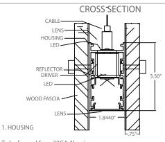
To be formed from 20GA Aluminum Finish: Baked white enamel (standard) Direct / Indirect Lighting (standard) All fixtures are pre-wired All steel parts are phosphate treated for corrosion resistance before painting procedure and then baked with superior adhesion for durability
