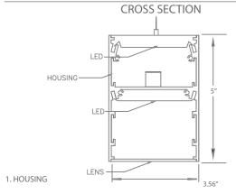
To be formed from 20GA Aluminum Finish: Baked white enamel (standard) Direct / Indirect Lighting (standard) All fixtures are pre-wired
