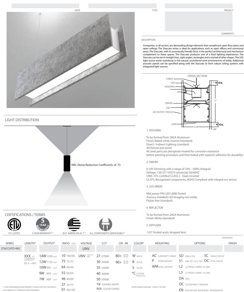
\* ALL INTERNAL PARTS ARE ACCESSABLE / SERVICEABLE (DRIVERS / LED BOARDS / OUICK CONNECTS)
