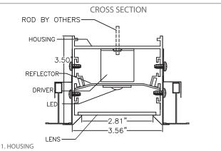
To be formed from extruded aluminum 6063t5 Finish: Baked white enamel (standard) Indirect Lighting (standard) All fixtures are pre-wired All steel parts are phosphate treated for corrosion resistance before painting procedure and then baked with superior adhesion for durability
